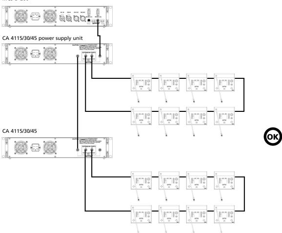
Set up the microphone stations as a branch or in a circle.
